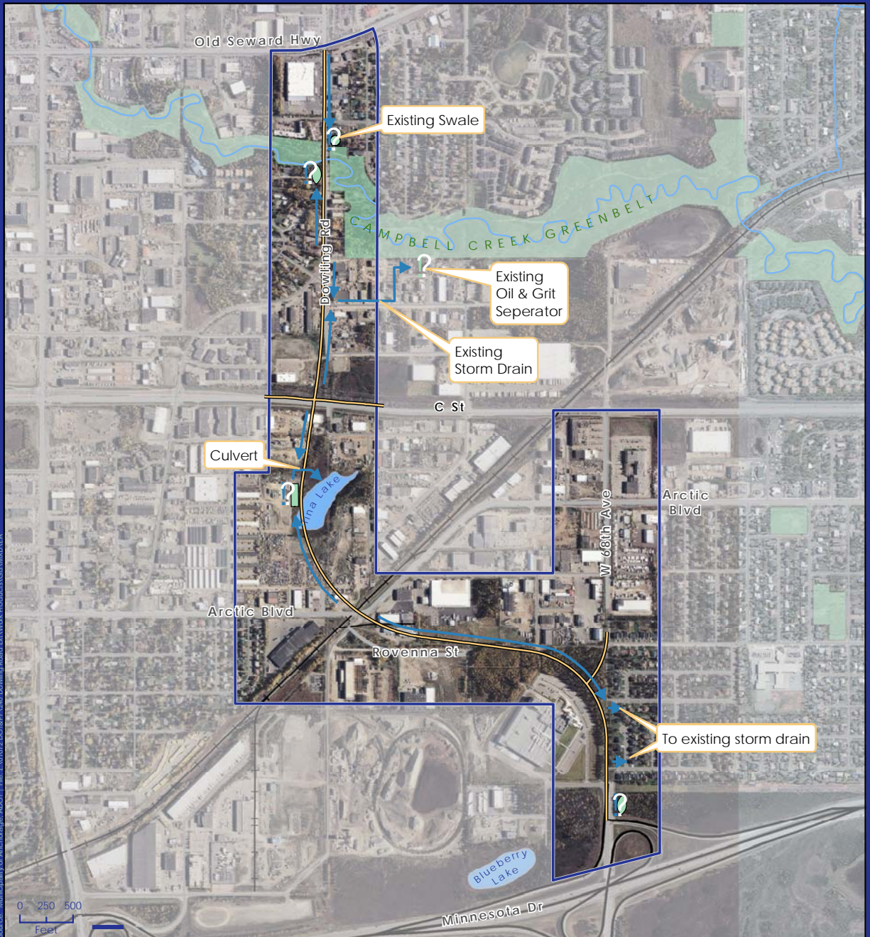
Figure 3.9 Approximate Location of Proposed Drainage Swales
